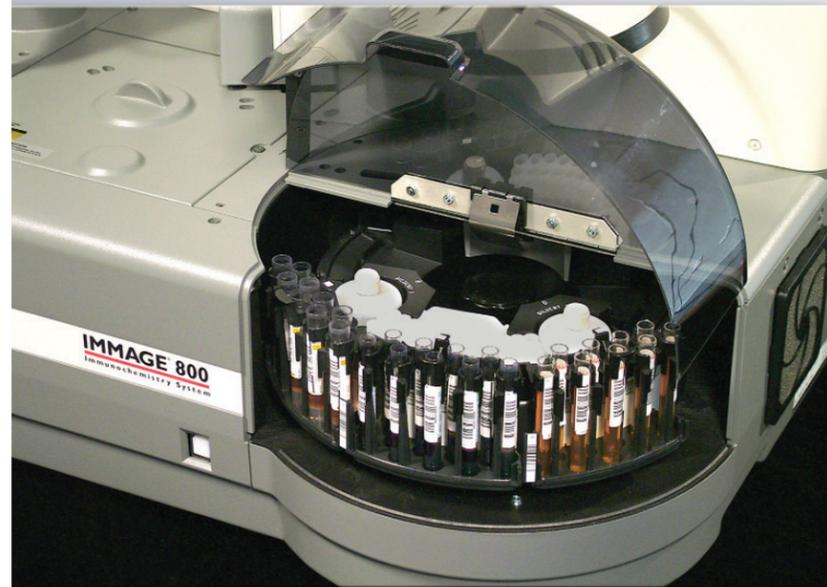
*The IMMAGE 800 provides utmost flexibility for disease state testing. It holds up to eight sample racks, accommodating up to 72 samples in a variety of containers.*
